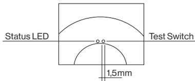
Note: Press test switch carefully to avoid damaging it.
